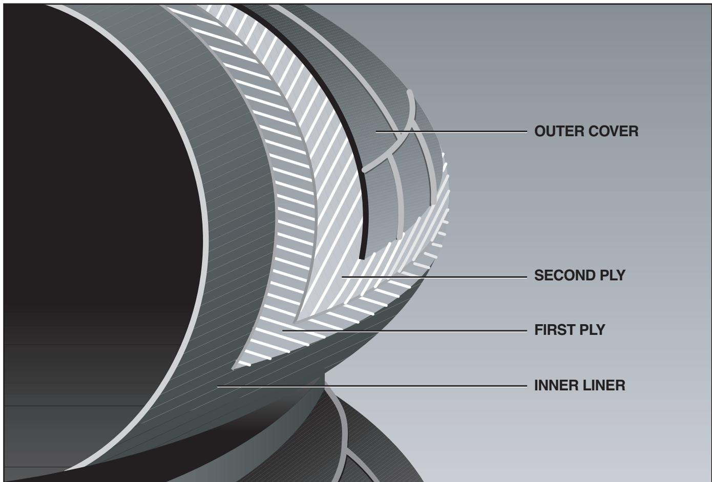
An air spring is a carefully designed rubber/fabric bellows which contains a column of compressed air. The rubber bellows itself does not provide force or support load. This is done by the column of air.
