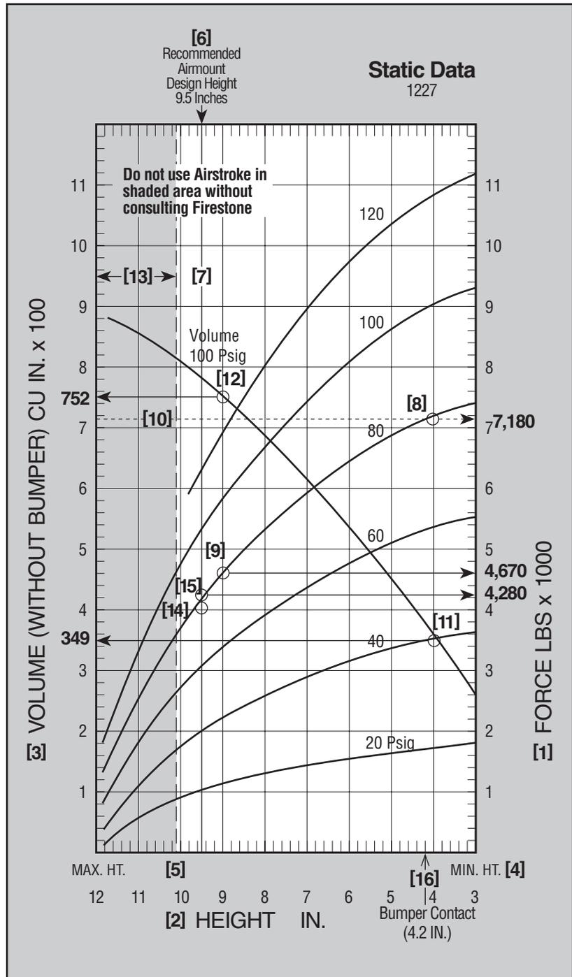
In the example the effective area of a #22, at 4.0 inches using the 80 psi curve, is:
