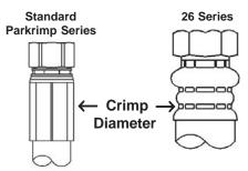
8b. Measure crimp diameter on the flat surfaces of the crimped shell, referenced in the above illustration. Reference crimp diameter on page C-26.
