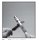
8a. Measure crimp diameter of each fitting at the top, middle and bottom of the shell. Take measurements at a minimum of three places around the shell circum-ference. Verify crimp diameter is within tolerances.
