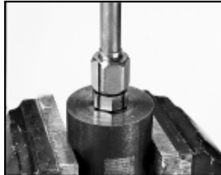
Fig. C15 — Fully tightened positioned with displaced mark
