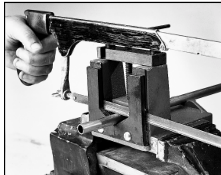
Fig. C4 — Parker's Tru-Kut sawing vise used with hacksaw
