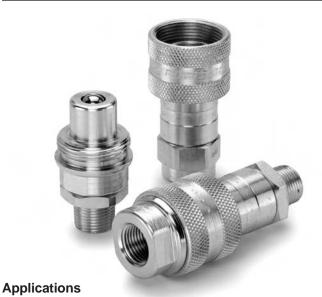
Parker 3000 Series couplings with their threaded union locking system and precision ball-type check valves, are designed for extreme high pressure applications such as found on portable hydraulic rams. See pages noted in Table of Contents for dust plugs and caps for the Parker full line of hydraulic couplings.
