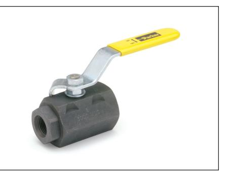
Parker's industrial ball valve product line is intended for general purpose use. Please be aware that ball valves are intended for use in the fully open or closed positions. Depending on application conditions, throttling of the valve may result in premature seal failure and/or inability to turn the valve handle.
