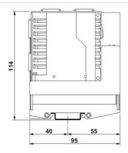
The illustration shows a version of the interface module with the head station FL SWITCH MM  $\ensuremath{\mathsf{HS}}$
