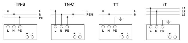
The connection for 100 V AC ... 240 V AC is made using the L, N and PE screw connections.
