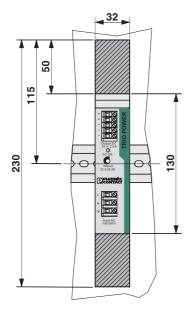
Mounting position: Installation depth 115 mm (+ DIN rail)
