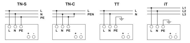
The connection for 100 V AC  $\dots$  240 V AC is made using the L, N and PE screw connections.
