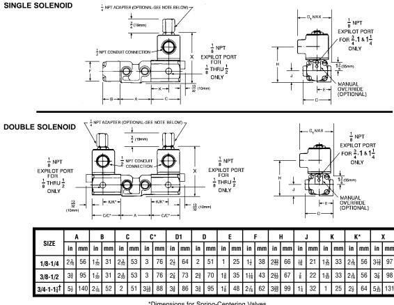
\*Dimensions for Spring-Centering Valves. NOTE: Adapter is supplied when specified, by adding suffix "-H" to product number
