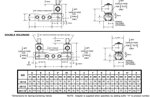
Refer to page V-44.1, under Body Detail, for port mounting hole locations for all valves shown above. †11/4" size valve has internal capacity of 11/4" (32mm) diameter. Sideported valves have 1" NPT ports; subplate for subplate mounting style has 11/4" NPT ports.
