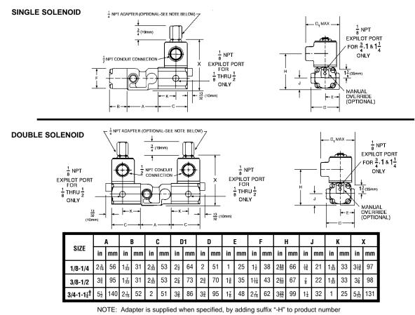
Refer to page V-24.1 under Body Detail, for port and mounting hole locations for all valves shown above. †11/4" size valve has internal capacity of 11/4" (32mm) diameter. Sideported valves have 1" NPT ports; subplate for subplate mounting style has 11/4" NPT ports.
