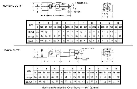
Refer to page V-24.1 under Body Detail, for port and mounting hole locations for all valves shown above.
