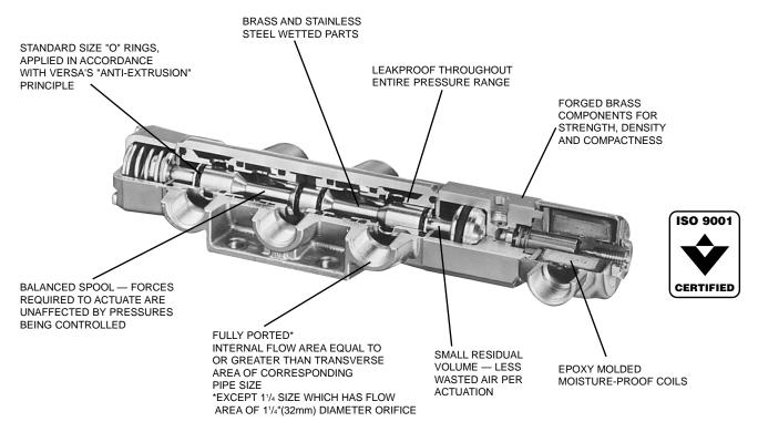
EVERY VALVE FUNCTIONALLY TESTED THROUGHOUT COMPLETE PRESSURE RANGE BEFORE SHIPPING
