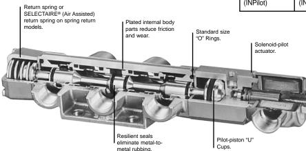
Cutaway shows side-ported "Oil-Free Service" Series "V" . . . one of many models in the complete Versa line. II. IF THE REQUIRED VALVE IS:
