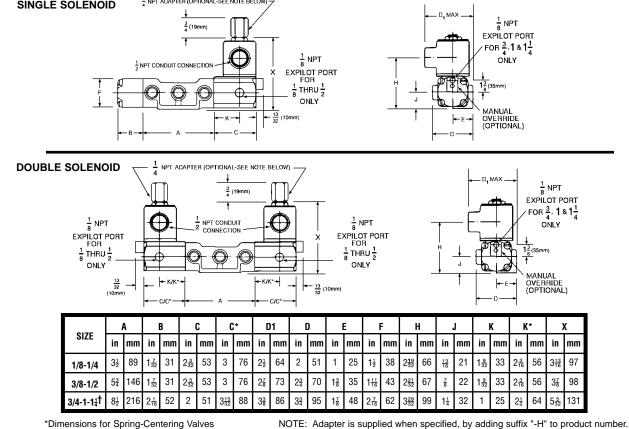
Refer to page V-54.1, under Body Detail, for port mounting hole locations for all valves shown above. †11/4" size valve has internal capacity of 11/4" (32mm) diameter. Sideported valves have 1" NPT ports; subplate for subplate mounting style has 11/4" NPT ports.
