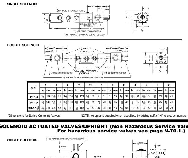
SOLENOID ACTUATED VALVES/UPRIGHT (Non Hazardous Service Valves. For hazardous service valves see page V-70.1.)
