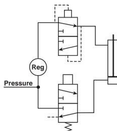
**Dual Pressure Actuation of Double Acting Cylinder**
