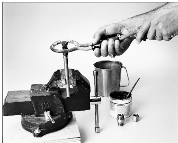
Fig. B5 — Multi-Flame Torch Brazing
